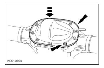
4. **NOTE:** Service refill capacities are determined by filling the axle to the bottom of the fill hole with the axle at ride height.
