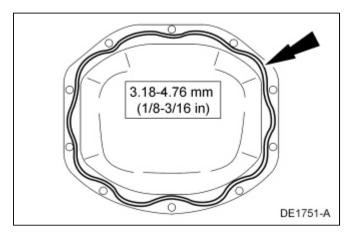
3. **NOTE:** The differential housing cover must be installed within 15 minutes of application of the silicone sealant, or new sealant must be applied. If possible, allow one hour before filling the axle housing with axle lubricant to make sure the silicone sealant has cured.
